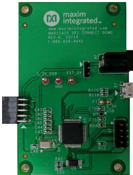
Figure 2: Communication Board: (MAXQ622: for USB to SPI communication from Laptop to ADC)
